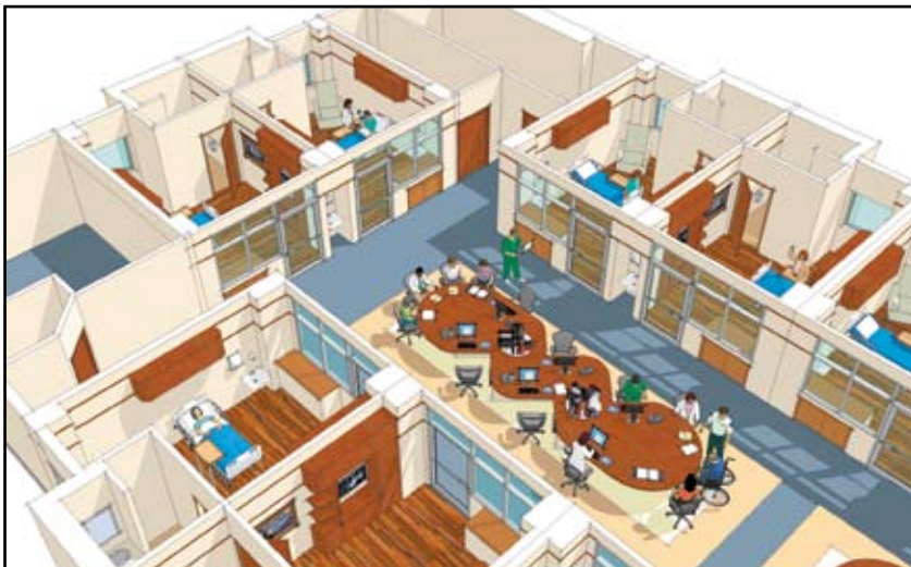
Figures 1 and 2. The plan for all patient care units in the North Georgia Medical Center features no corridors; the patient rooms wrap around a single clinical nursing worktable.
